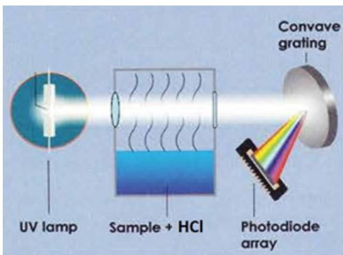
The measuring principle is based on the UV light absorption spectrum of Hydrogen Sulfide gas H<sub>2</sub>S in equilibrium with dissolved Hydrogen Sulfide gas in water sample.
